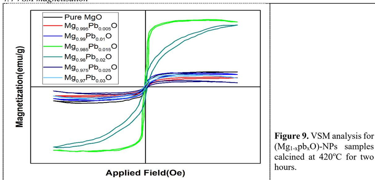
The magnetisation behaviour curves for the prepared nanocrystallites ( $\text{Mg}_{1-x}\text{pb}_x\text{O}$ ) samples were created by modifying the Pechini method and calcined at  $420^\circ\text{C}$  for two hours, as plotted in Figure 9. The samples were investigated by vibrating samples magnetometer (VSM). The VSM shows the hysteresis loops for the seven samples examined at room temperature and motivated by defects.
