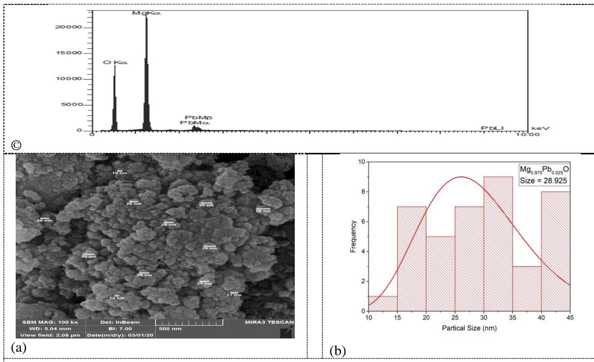
**Figure 7.** FE-SEM test analysis for  $Mg_{0.975}Pb_{0.025}O$  sample. (a) FE-SEM for  $Mg_{0.975}Pb_{0.025}O$  sample. (b) Histogram for  $Mg_{0.975}Pb_{0.025}O$  sample. (c) EDS for  $Mg_{0.975}Pb_{0.025}O$  sample.
