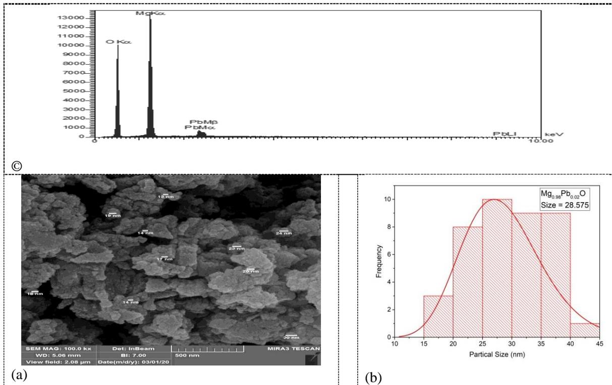
**Figure 6.** FE-SEM test analysis for  $Mg_{0.98}Pb_{0.02}O$  sample. (a) FE-SEM for  $Mg_{0.98}Pb_{0.02}O$  sample. (b) Histogram for  $Mg_{0.98}Pb_{0.02}O$  sample. (c) EDS for  $Mg_{0.98}Pb_{0.02}O$  sample.
