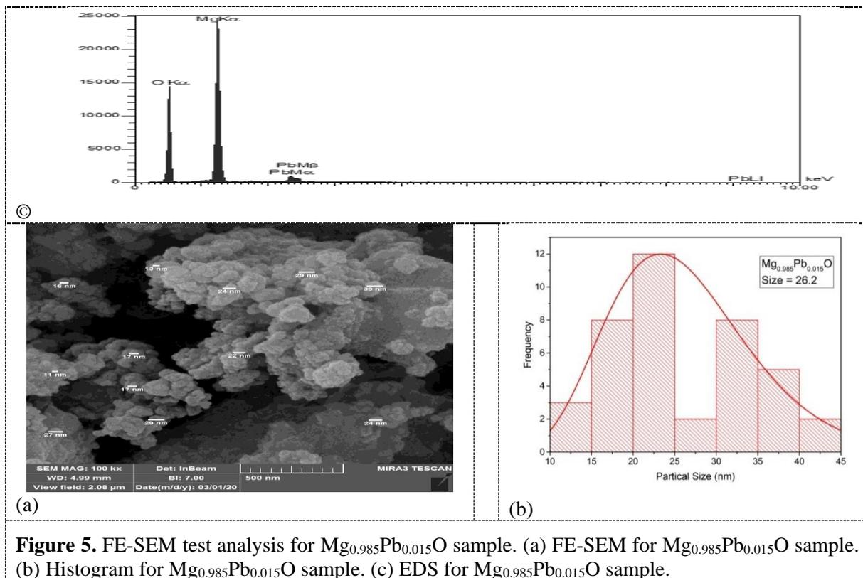
**Figure 5.** FE-SEM test analysis for  $Mg_{0.985}Pb_{0.015}O$  sample. (a) FE-SEM for  $Mg_{0.985}Pb_{0.015}O$  sample. (b) Histogram for  $Mg_{0.985}Pb_{0.015}O$  sample. (c) EDS for  $Mg_{0.985}Pb_{0.015}O$  sample.
