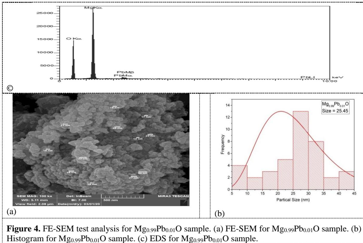
**Figure 4.** FE-SEM test analysis for  $Mg_{0.99}Pb_{0.01}O$  sample. (a) FE-SEM for  $Mg_{0.99}Pb_{0.01}O$  sample. (b) Histogram for  $Mg_{0.99}Pb_{0.01}O$  sample. (c) EDS for  $Mg_{0.99}Pb_{0.01}O$  sample.
