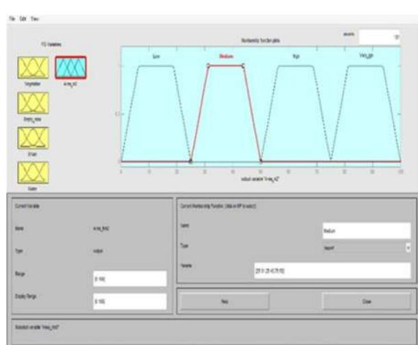
**Figure 5.** Membership function editor for input. **Figure 6.** Membership function editor for output.
