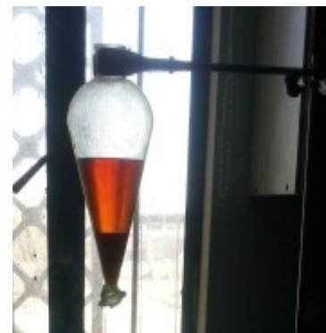
Fig. 2 : Separating funnel apparatus for phenolics.
