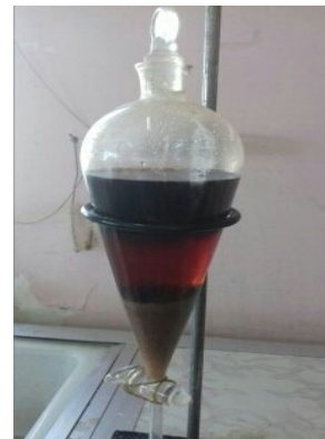
Fig. 1 : Separating funnel apparatus for alkaloids.
