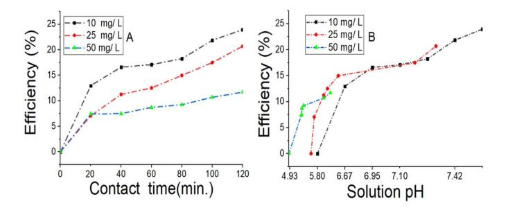
**Fig.3** shows the Nickle (II) removal efficiency (%) from aqueous solution (A) for many contact times (*min.*), and (B) different solution pH, with the initial concentration (10-50 mg/L).
