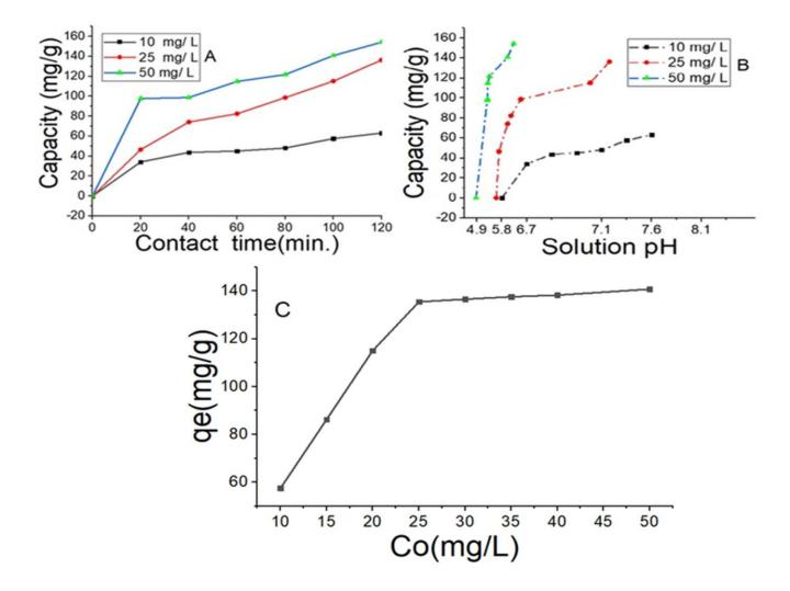
**Fig.4** shows the Nickle (II) adsorption capacity (mg/g) (A) for many contact times (min.), (B) different solution pH, and (C) the initial concentration (10-50 mg/L).
