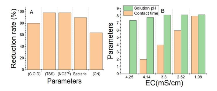
**Fig.7** (A) Reduction rate percentages of the Al-Muaymira wastewater parameters - Iraq after eight hours' treatment with present composite Nano-fibers film, Parameters such as solution pH and periods contact time as a function of electrical conductivity of wastewater after treatment by  $\gamma$ -Fe2O3-PAN nanofibers.
