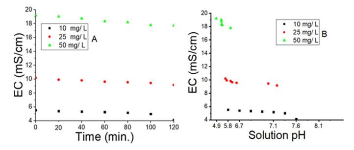
**Fig.5** shows the electrical conductivity (mS/cm) before and after adsorption of Nickle (II) from the aqueous solution by composite nanofibers (A) for many contact times (min.), and (B) different solution pH, with the initial concentration (10-50 mg/L).
