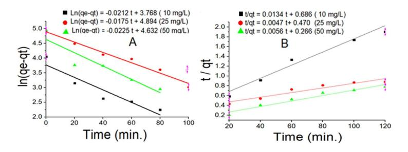
**Fig.6** Adsorption kinetics of Nickle (II) on composite  $\gamma$ -Fe2O3-PAN nanofibers by using (A) the pseudo first- order model which represented by relation between *ln* (*qe*-*qt*) against *t*, (B) Pseudo-second-order model which is represented by relation *t/qt* against *t*, when increasing initial concentrations of aqueous solution (*10-50 mg/L*).
