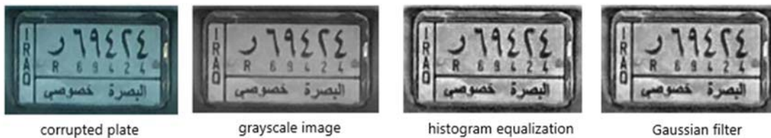
FIGURE 7. Results of the first two steps in the suggested method for recognizing the characters.
