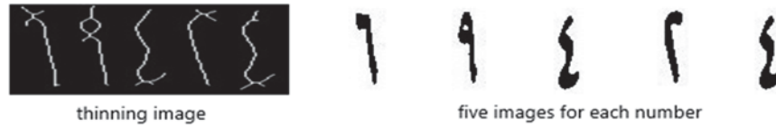
FIGURE 10. Results of thinning image and separation of numbers in the image.
