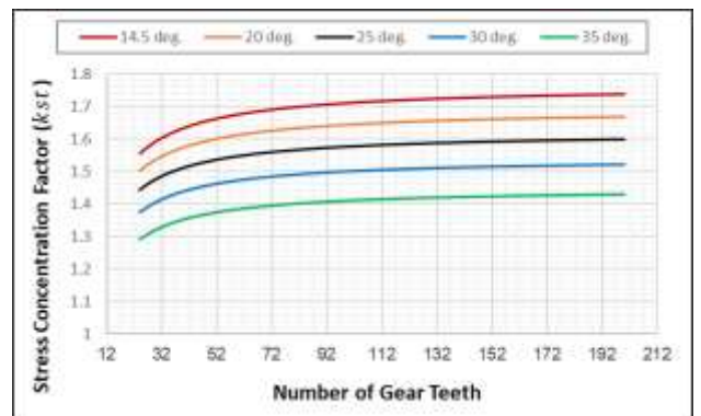
Figure 19. The effect of the gear module on the value of the Stress Concentration Factor (Kst).
