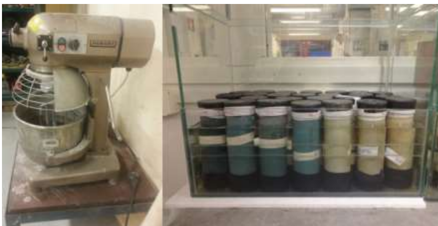
Figure 2: Laboratory mixer and curing specimens aimed for UCS and consistency limits tests
