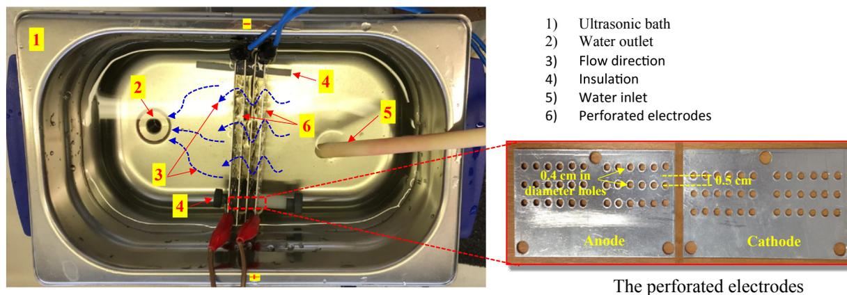
Fig. 1. The U-E reactor.
