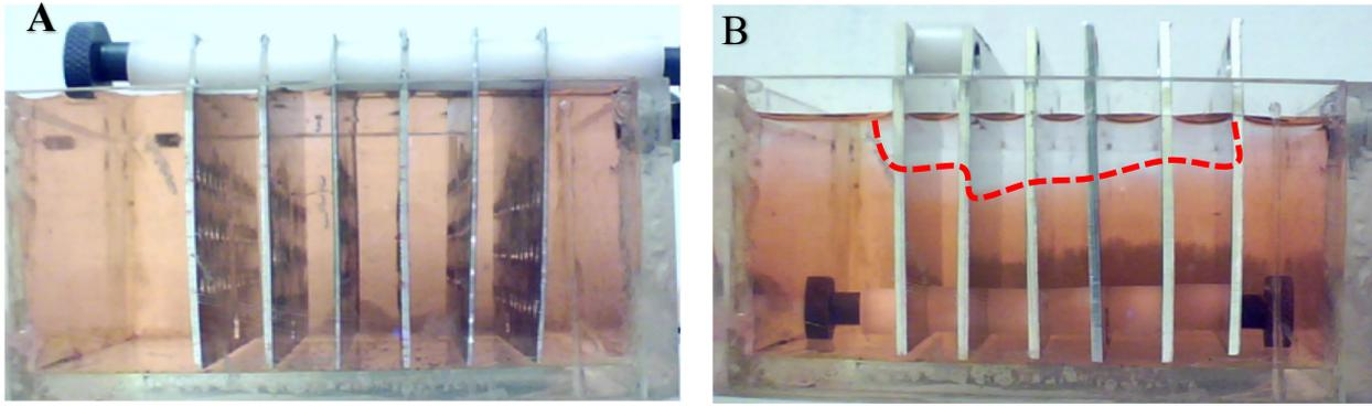
Fig. 2. Mixing efficiency of (A) new EC electrodes, (B) A traditional EC electrodes.
