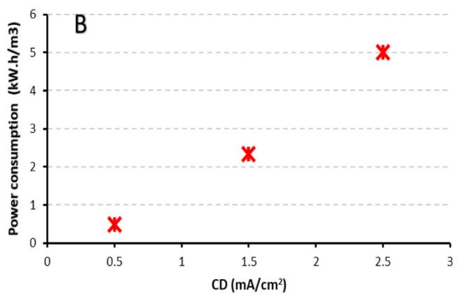
Fig. 4. Effect of CD on: (A) *E.coli* inactivation, (B) Power consumption.
