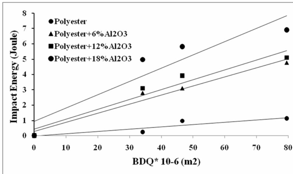
Fig. 4: Illustrate the relation between impact energy and BDΦ
