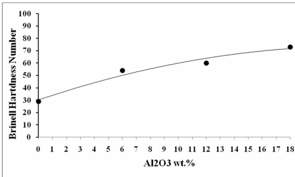
Fig. 3: Illustrate the relation between concentration of  $\alpha$ -alumina fibers and Brinell hardness number.
