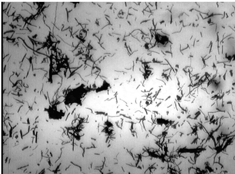
**Figure 1: Light optical microscopy images of chopped alumina fibers which prepared in this work(Magnification 400X).**
