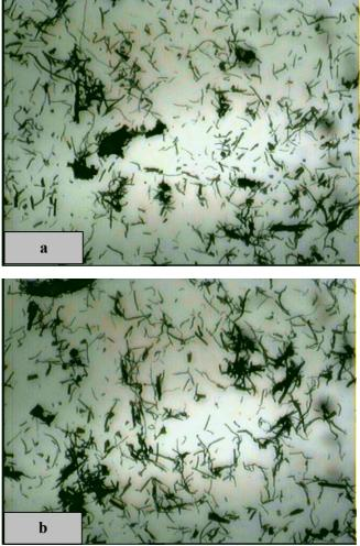
Figures 1a and b: Light optical microscopy images of chopped alumina fibers which prepared in this work(Magnification 400X).
