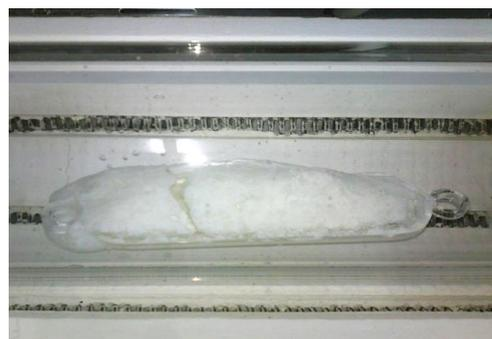
Figure 3. Ionic liquid surface blocked
