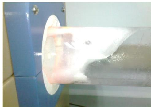
Figure 4. Quartz tube partially contaminated
