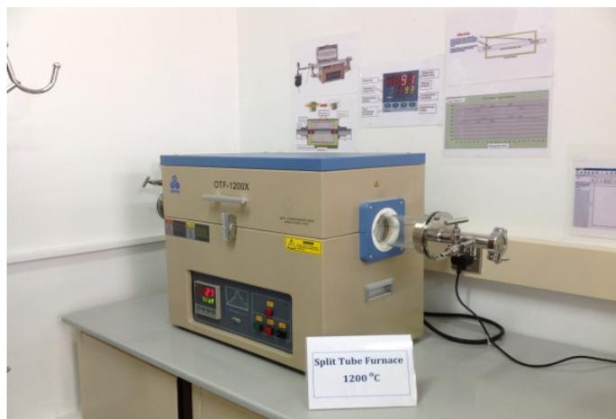
Figure 1. Split tube furnace
