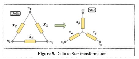
Compare the three components of delta with three components of star, then applying the equations (1) and (3) to get three relations:
