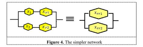
By apply equation (1) on the left diagram of figure 4 we find  $x_{rr1} = x_1 x_{r1}$  and  $x_{rr2} = x_2 x_{r2}$  which are implies to  $R_{rr1} = R_1 R_{r1}$  and  $R_{rr2} = R_2 R_{r2}$ . Then from equations (7) and (8) we get:
