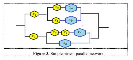
By apply equations (1) and (3) for the network in figure 3 to get  $x_{r1} = 1 - (1 - x_3 x_a)(1 - x_4 x_b)$  and  $x_{r2} = 1 - (1 - x_a)(1 - x_3 x_4 x_b)$ So,  $R_{r1} = 1 - (1 - R_3 R_a)(1 - R_4 R_b)$  and  $R_{r2} = 1 - (1 - R_a)(1 - R_3 R_4 R_b)$ . Then we get  $R_{r1} = R_3 R_a + R_4 R_b - R_3 R_4 R_a R_b$  (7)  $R_{r2} = R_a + R_3 R_4 R_b - R_3 R_4 R_a R_b$  (8) Journal of Physics: Conference Series
