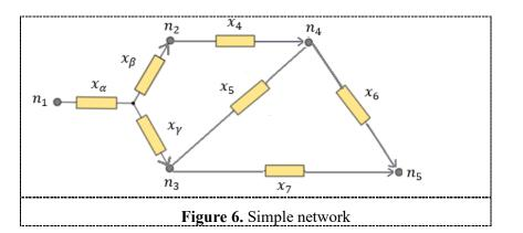
Now applying the reduction method on the subnetwork resulting from deletion  $x_{\alpha}$  from figure 6. The minimal paths of this subnetwork are  $P_1 = \{x_{\beta}x_4x_6\}, P_2 = \{x_{\beta}x_4x_5x_7\}, P_3 = \{x_{\gamma}x_7\}$ , and  $P_4 = \{x_{\gamma}x_5x_6\}$ , so that this subnetwork converts to a series- parallel subnetwork and can drown as in figure 7
