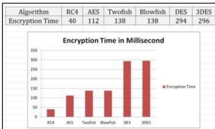
Figure (4) : Encryption Time for proposed algorithms.
