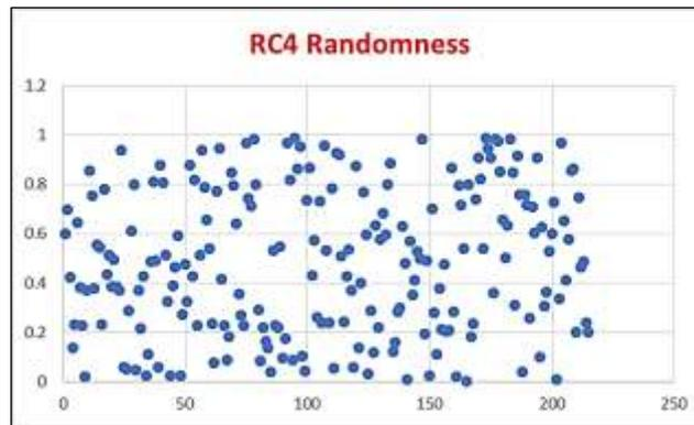
**Figure (9) : P-values For RC4 – Ciphertext.**
