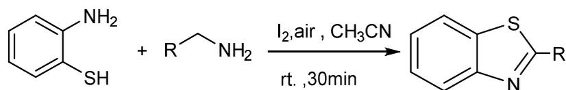
R= Ph, 4-OCH<sub>3</sub>-Ph, 4-Cl-ph, 3,4-Cl-Ph, 4-F-ph, 4-CH<sub>3</sub>-Ph, 4-OCF<sub>3</sub>-Ph
