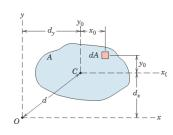
The second integral is zero, since  $\int (y_0)dA = A\bar{y}_0$  and  $\bar{y}_0$  is automatically zero with the centroid on the  $x_0$ -axis.
