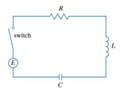
It is known from physics that the voltage drops across the resistor, inductor, and capacitor are: RI,  $L\frac{dI}{dt}$  and  $\frac{Q}{C}$  respectively. Kirchhoff's voltage law says that the sum of these voltage drops is equal to the supplied voltage
